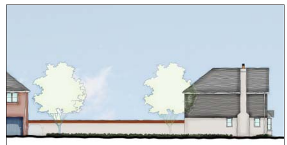
5.2. Proposed Wychert Wall by the entrance of Stanbridge Road
