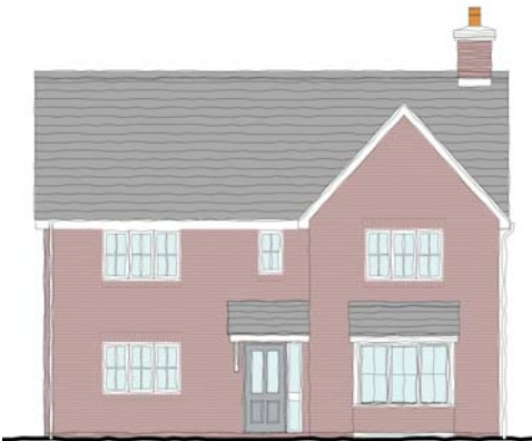
Plot 22: Character Features Rooftop chimney, cross-bar windows, brick cladding, voussoir lentils, brick sill, lean-to porch
