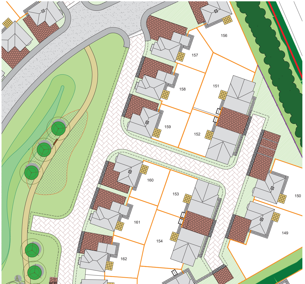
9.1. Extract of External Works Plan showing the changes in material on the streets and road surfaces
