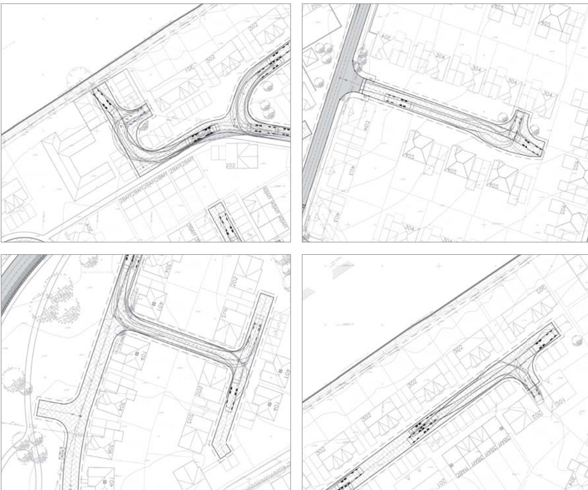
9.3. Swept Path Analysis. Extract of proposed site plan indicating tracking for anticipated manoeuvres
